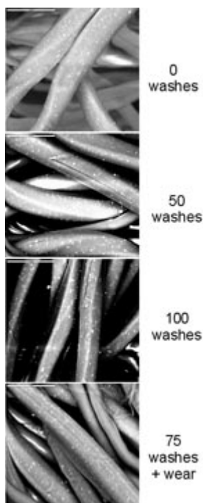
Figure 1. Socks containing 12% copper impregnated fibers were washed up to 100 consecutive times by using AATCC test method (TM) 150. The copper impregnated fibers were analyzed by scanning electronic microscope (SEM). The amount of copper particles throughout the fibers was not changed. Moreover, as shown in the lower SEM picture, there was no reduction in copper oxide particles in socks used and worn 75 times.
