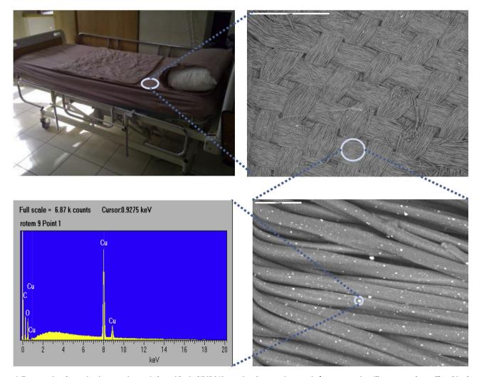
**Figure 1.** Two scanning electronic microscope images (taken with a Jeol JMS 840 scanning electron microscope) of a representative pillowcase are shown. The white dots are the copper oxide particles embedded in the polyester fibers. The chart is an X-ray photoelectron spectra analysis (done with a Shimadzu XRD 6000, TN-5500 X-ray analysis system) of the encircled white dot, showing a peak at 8 KeV corresponding to copper.
