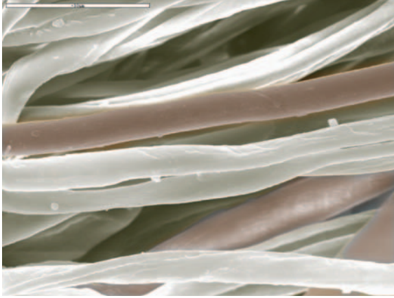
FIGURE 2. Mixture of cotton copper oxide plated fibers and untreated fibers as observed by SEM.
