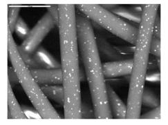
Fig. 1 Scanning electronic microscope picture of copper oxide impregnated polyester yarn used in the tested socks. The white dots are copper oxide particles.
